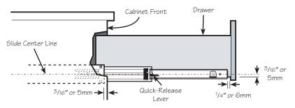
3. Screw the cabinet slide member to the cabinet with the supplied screws. The screws should land on the center line drawn previously. As shown in the diagram, the front of the slide should be 3/16" or 5mm from the front of the cabinet. (These distances assume that the drawer will have a false front that overlays the cabinet.) Start by driving the screws in the horizontal slots closest to the front and back of the cabinet. Use only two screws at this point.
